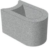
Length: 400mm Width: 250mm Height: 250mm Per m<sup>2</sup>: 390kg Weight per Unit: 30kgs Pallet Quantity: 48
