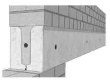
**3 KWIKLIN**Designed to create a bearer beam for heavy duty applications. Laminated bearer beam assembly with a minimum width of 210mm
